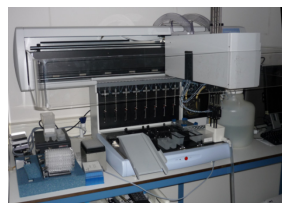
Robotic liquid handling system for automated enzyme / immunochemical assays
